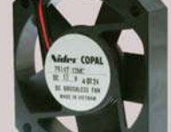
F614T ● Air flow: 0.36, 0.43 m 3 /min ● Static pressure: 20, 29 Pa ● Noise: 23, 29 dB(A) ● Rated voltage: 5, 12, 24 VDC ● Dimensions: □62×14.5 mm
