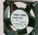
F410T ● Air flow: 0.11, 0.15 m 3 /min ● Static pressure: 10, 23 Pa ● Noise: 12, 18 dB(A) ● Rated voltage: 5, 12 VDC ● Dimensions: □40×10 mm
