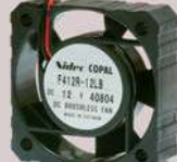
F412R ● Air flow: 0.11, 0.15 m 3 /min ● Static pressure: 15, 26 Pa ● Noise: 16, 23 dB(A) ● Rated voltage: 5, 12, 24 VDC ● Dimensions: □41×12.2 mm
