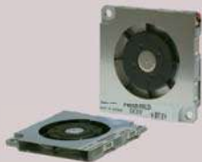
F455B (Side flow type) ● Air flow: 0.28 m 3 /min ● Static pressure: 20, 30, 47 Pa ● Noise: 20 dB(A) ● Rated voltage: 5 VDC ● Dimensions: □45×5 mm
