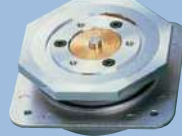
PD60ER ● Mirror size: φ72 mm ● Dynamic pyramidal angle error accuracy 60/30 sec. ● Speed range 5000~12000 r/min. ● For digital PPCs, digital photo labs
