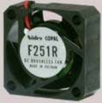
F251R ● Air flow: 0.04, 0.05, 0.06 m 3 /min ● Static pressure: 20, 30, 47 Pa ● Noise: 11, 15, 20 dB(A) ● Rated voltage: 5, 12 VDC ● Dimensions: □25×10 mm
