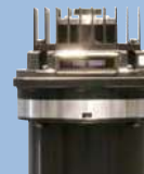
PV60SRG ● Mirror size: φ50~70 mm (t=3 to 5mm) ● Dynamic pyramidal angle error accuracy 30 sec. (peak to peak) ● Speed range 55000~70000 r/min. ● For Semiconductor Inspection, Non-Destructive Inspection, etc
