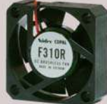
F310R ● Air flow: 0.06, 0.09 m 3 /min ● Static pressure: 14, 23 Pa ● Noise: 13, 17 dB(A) ● Rated voltage: 5, 12 VDC ● Dimensions: □30×10 mm
